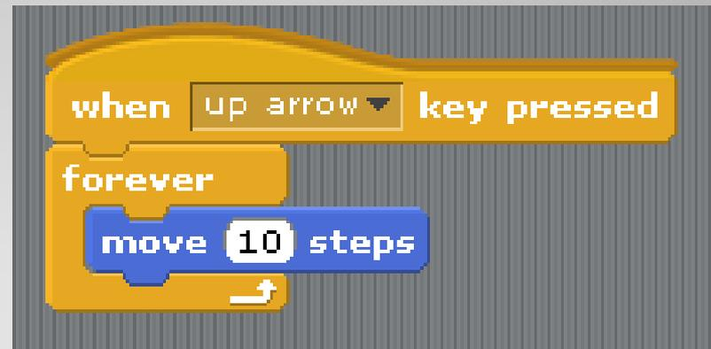
When the up arrow is pressed it will continuously move forward by 10 steps
