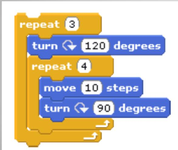
The outer loop causes the 4 passes of the inner loop to be completed 3 times.
